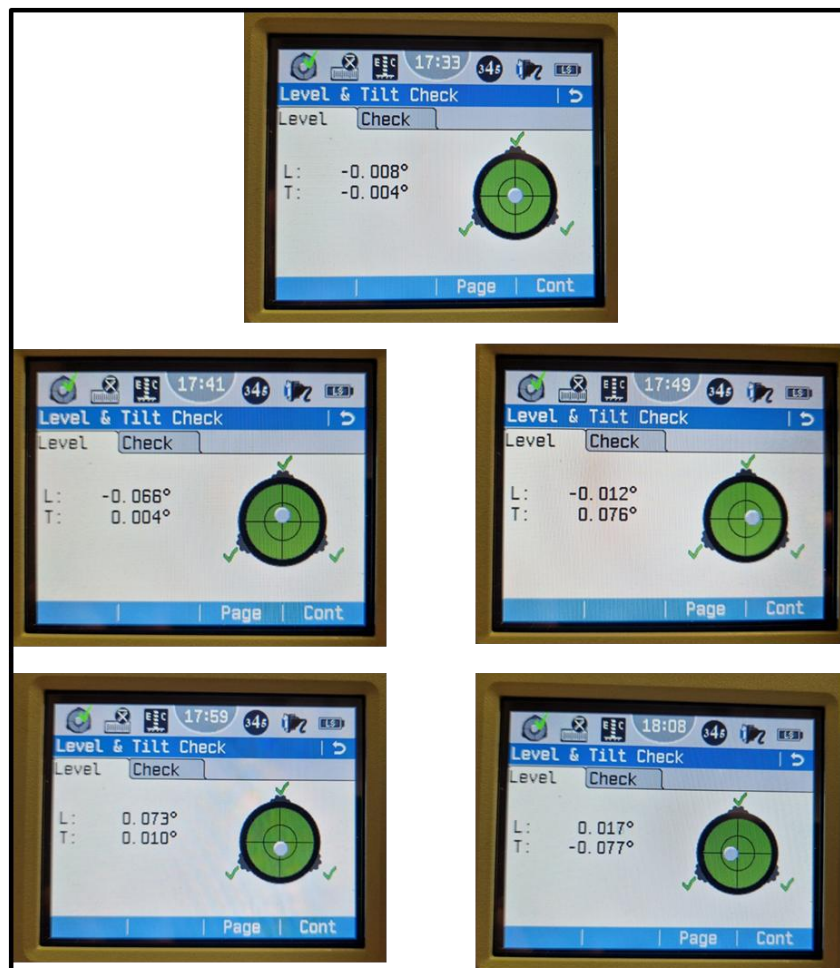
Figure 1. The positions of level's bubble during measurements
